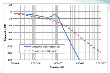
**Figure 1:** Typical Common Mode and Differential Mode Attenuation provided by the filter as a function of frequency when using parts suggested in the "Typical Connection Diagram". Source and load resistance are  $50\Omega$ .
